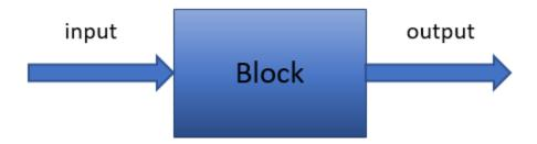
A block can represent a physical component, a small system, or a function; an input/output relationship fully characterizes the block. Consider these examples:
